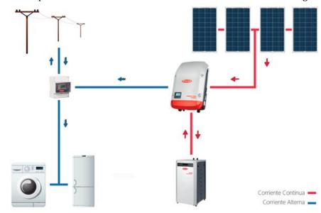
• Self-consumption with accumulation: It is the type of installation where the batteries charging or discharging, is managed by additional equipment, and the surplus energy production is discharged in batteries till the time is more useful.
