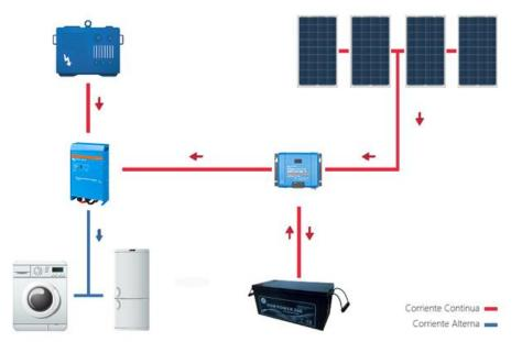
In this kind of installation, the regulator charges the battery with the energy generated by the panel or by direct current, and an inverter is needed to remove the energy stored in the battery by the regulator.
