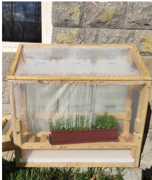
Figure 13 Foil tent with heat storage medium and water balloons
